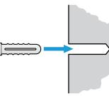
On **wood** or **siding**, you can skip this part and screw the bracket directly onto your wall.
