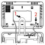
Secure the back plate to the wall, then loop the hang strap over the strain relief hook (Ĭ) Run the antenna through the hole (2)
