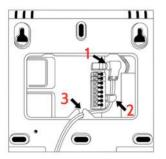
Plug in the power supply (1) and then clip the wire to the retainer clip (2) then into the strain relief hook (3)
