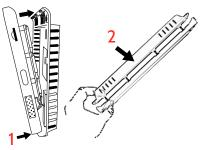
Place the panel onto the bottom of the back plate (1) and hinge upward and snap in place (2). Take care as you route the antenna into the wall
